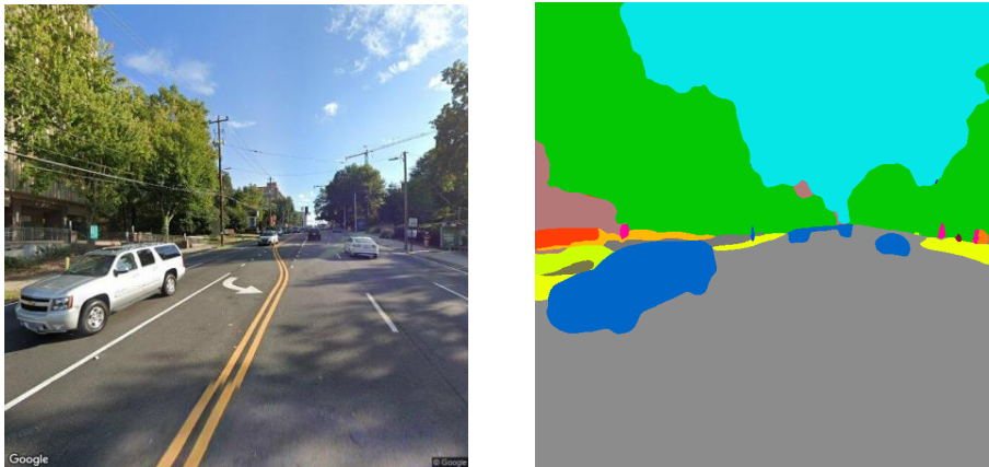
Figure 2. Street View image from Google API (left) and the result of image parsing using PSPNet (right)
